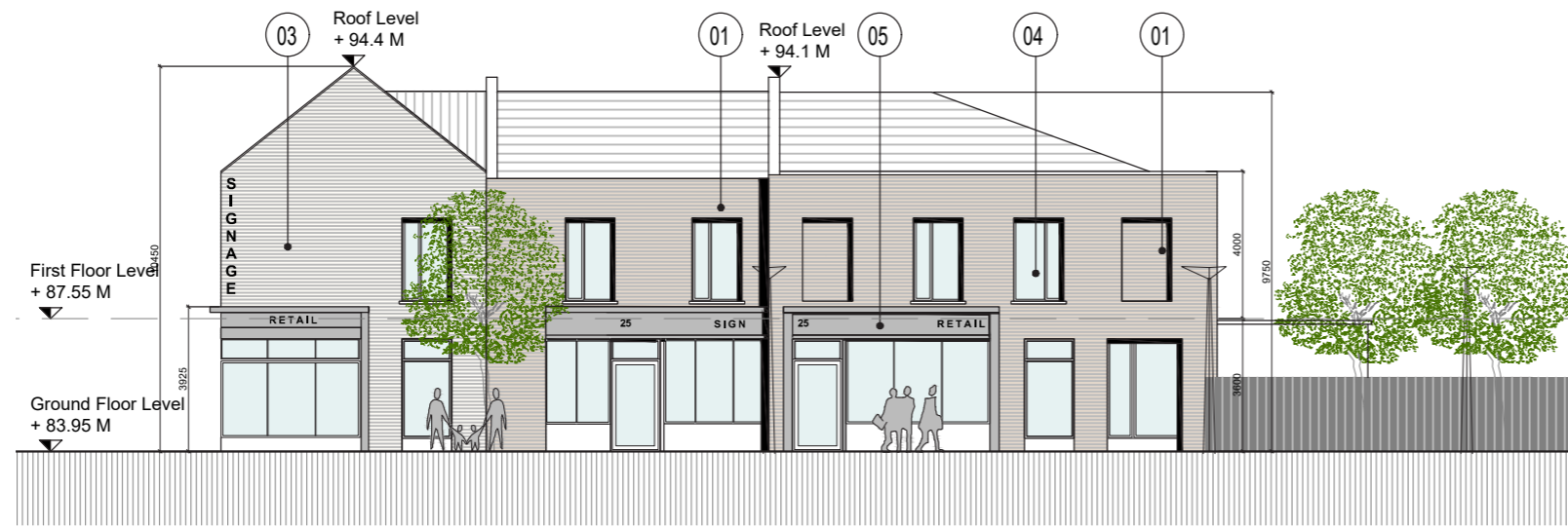
Block D2 - South Elevation
